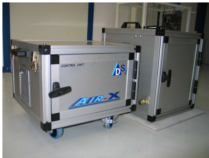
Special configuration for tilt test beds: The hydraulic unit (right hand box) is separated from the control unit for more compactness
