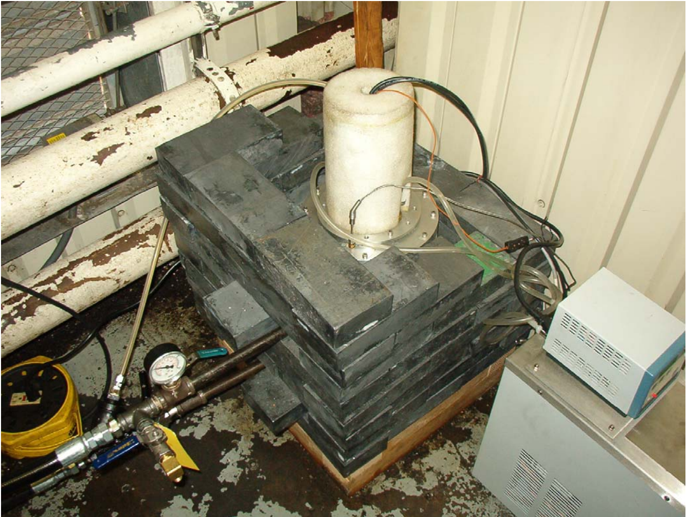
Figure 13: Flow-Through Reservoir in Lead Shield for Heavy-Duty Diesel Engines
